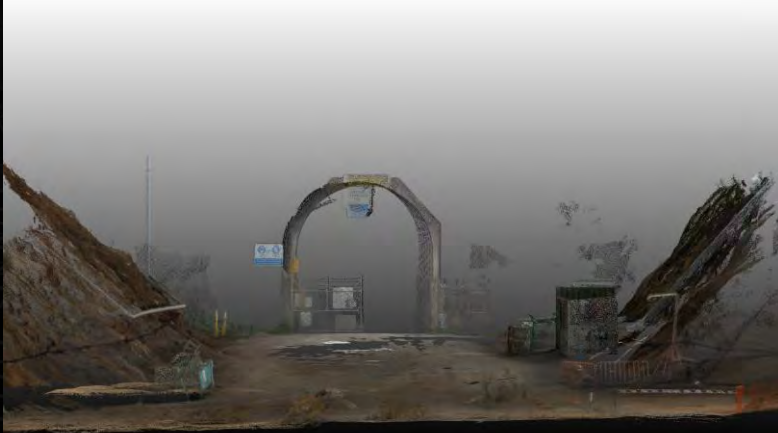
Colorised Point Cloud at Mine Portal
